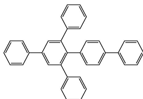
In a preferred embodiment of the invention, the organic enhancement layer may include an aromatic hydrocarbon having the following structure:
