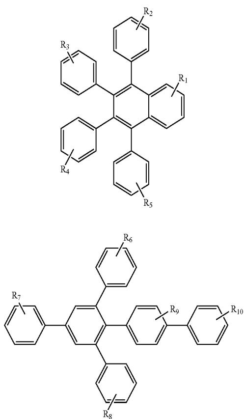
wherein R<sub>1</sub>–R<sub>10</sub> each represent no substitution, mono-, di-, or tri-substitution, and wherein the substituents are the same or different, and each is selected from the group consisting of alkyl, alkenyl, aryl, heteroalkyl and substituted aryl groups.
