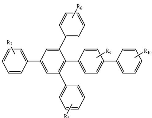
Such that R<sub>6</sub>–R<sub>10</sub> each represent no substitution, mono-, di-, or tri-substitution, and wherein the substituents are the same or different, and each is selected from the group consisting of alkyl, aryl, heteroalkyl, substituted aryl, substituted heteroaryl and heterocyclic groups.
