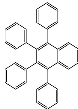
In another preferred embodiment of the invention, the organic enhancement layer may include an aromatic hydrocarbon having the following structure:
