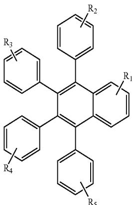
Such that R<sub>1</sub>–R<sub>5</sub> each represent no substitution, mono-, di-, or tri-substitution, and wherein the substituents are the same or different, and each is selected from the group consisting of alkyl, aryl, heteroalkyl, substituted aryl, substituted heteroaryl and heterocyclic groups
